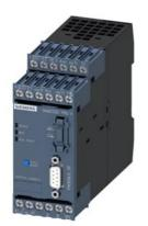
Basic unit SIMOCODE pro V PB PROFIBUS DP interface 12 Mbit/s, RS 485, 4I/3O freely parameterizable, Us: 110...240 V AC/DC, input for thermistor connection Monostable relay outputs, expandable by extension modules
