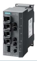
\*\*\*\*\*\*\*\*\*\* spare part \*\*\*\*\*\*\*\* SCALANCE X204-2FM, FO monitoring managed IE switch, 4x 10/100 Mbit/s RJ45 ports, 2x 100 Mbit/s multimode BFOC, LED diagnostics, error signaling contact with set pushbutton, redundant power supply, PROFINET IO device, network management, can be operated in redundant ring, incl. electron. manual on CD-ROM, C-plug optional.
