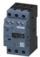
Circuit breaker size S00 for motor protection, CLASS 10 A-release 0.35...0.5 A N-release 6.5 A Screw terminal Standard switching capacity with transverse auxiliary switch 1 NO+1 NC
