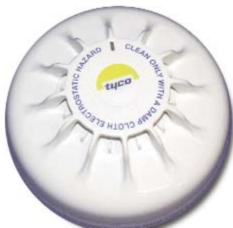
The detector is designed to transmit to a remote MINERVA® MX fire controller, digital signals which represent the status of the Carbon Monoxide and heat elements of the detector. Software within the controller is used to interpret the returned Carbon Monoxide and heat values to raise an alarm or other appropriate response according to the type of detector configured in 'MXCONSYS'.
