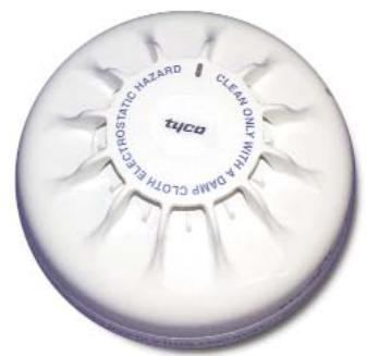
The detector is designed to transmit to a remote MINERVA® MX fire controller, digital signals which represent the status of the heat element of the detector. Software within the controller is used to interpret the returned heat values to raise an alarm or other appropriate response according to the type of detector configured in 'MXCONSYS'.
