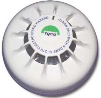
The detector is designed to transmit to a remote MINERVA® MX fire controller, digital signals which represent the status of the optical smoke and heat elements of the detector. Software within the controller is used to interpret the returned optical and heat values to raise an alarm or other appropriate response according to the type of detector configured in 'MXCONSYS'.
