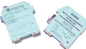
The EXI800 can detect a short circuit on the left-loop, the right-loop, or the IS loop and will isolate the offending loop connections from the other loop connections. The IS loop output of the EXI800 interfaces with the Pepperl+Fuchs KFDO-CS-Ex1.54 Galvanic Isolator, supplying loop voltage and signalling currents to the Intrinsically Safe loop.
